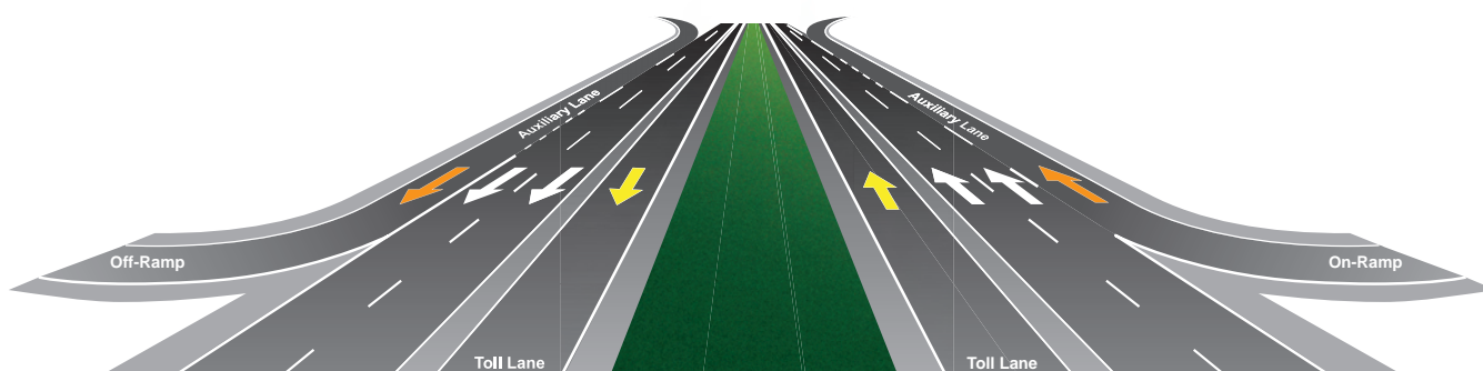
Proposed C-470 Interim - 1 Tolled Express Lane in each direction plus 2 General Purpose Lanes in each direction with Auxiliary Lanes (select locations)
